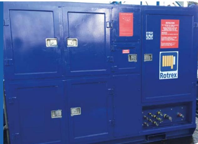
This range of Rotrex engineered hydraulic power units are Zone 2 certified and comply with British/European, ATEX and IEC standards.
