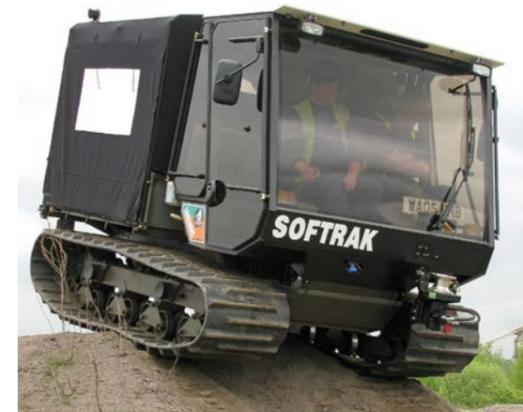
The Rotrex Softrak ATV is the foremost in low ground pressure machines available for hire. It is able to traverse steep slopes as a result of its exceptional ground clearance and low centre of gravity.
