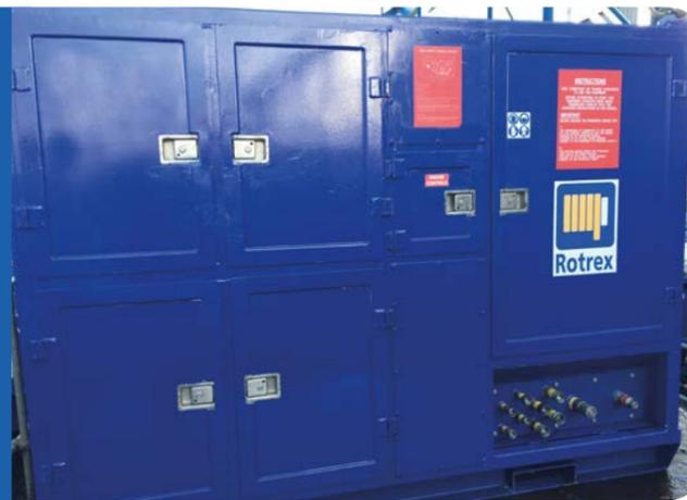
This range of Rotrex engineered hydraulic power units are Zone 2 certified and comply with British/European and IEC standards.
